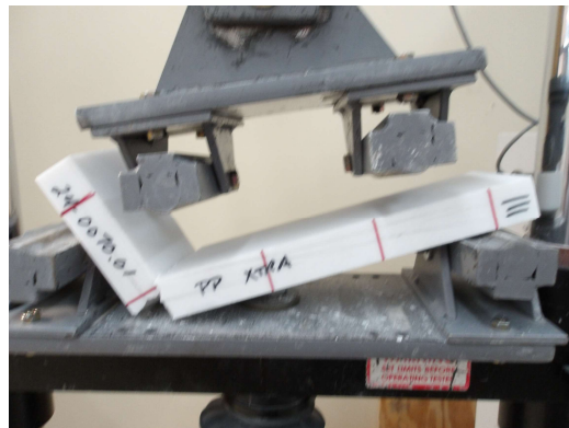
Photo No. 8 ASTM C880 – Representative Specimen Failure Mode (Perpendicular Loading)
