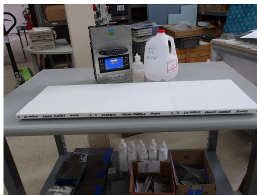
Photo No. 14 ANSI A326.3 – Dynamic Coefficient of Friction Test Set Up
