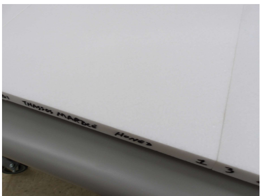
Photo No. 15 ANSI A326.3 – Specimen Detail (Honed Finish Depicted)
