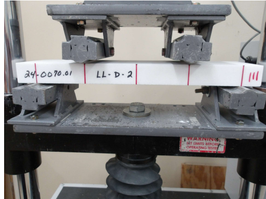
Photo No. 6 ASTM C880 – Load Application Fixture Detail
